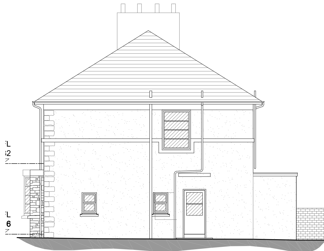
Side elevation - as existing
